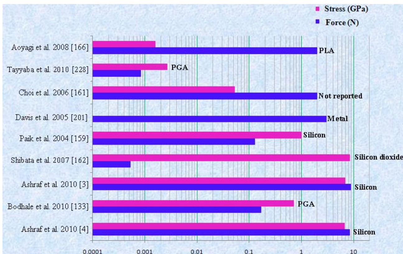
Figure 24. Comparison of force versus stress on microneedles.
