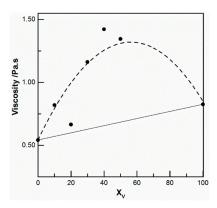
**Figure 1.** Variation of the viscosity of chitosan CS-102/ PEO (M = 1000 kg/mol) mixtures in 0.5 M acetic acid at  $0.5 \, \mathrm{s^{-1}}$  as a function of weight fraction of PEO ( $X_v$ ). Total polymer concentration  $5\% \, w/v$ . PEO: poly(ethylene oxide); CS: Chitosan.
