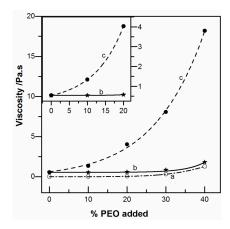
**Figure 2.** Variation of the viscosity at  $0.5 \text{ s}^{-1}$  of added PEO (M = 1000 kg/mol) expressed in percent of total polymer concentration in the mixtures. (a) PEO solution in 0.5 M acetic acid O; (b) additivity calculated for each values of "a" added into pure chitosan CS- $102 \times \text{ and (c)}$  blends chitosan CS- $102 \times \text{ PEO}$  as a function of the weight fraction of PEO ●.
