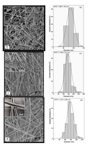
**Figure 3.** Representative SEM images and fiber diameter distributions of the electrospun nanofibers obtained from blend of powdered PEO into chitosan solutions (CS/PEO) at weight ratio (a) 90/10; (b) 80/20; (c) 70/30; and (d) 60/40. The insets show the high magnification images. The fiber diameter distributions of each are shown on the right. AFD: average fiber diameter; SEM: scanning electron microscopy.
