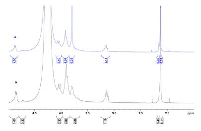
**Figure 5.**  $^{1}$ H-NMR spectrum for the CS-102/PEO (80/20) mixture solubilized in 0.5 M acetic acid with added D<sub>2</sub>O (**A**) and CS-102 solubilized in 0.5 M acetic acid with added D<sub>2</sub>O (**B**).
