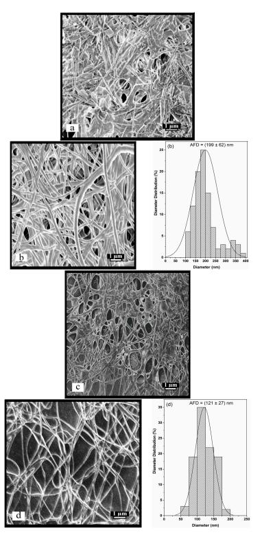
**Figure 4.** The SEM images of the membrane surface of chitosan/PEO at different ratios. (a) 60/40 neutralized in water; (b) 60/40 neutralized in ethanol/water mixture; (c) 80/20 neutralized in water; and (d) 80/20 neutralized in ethanol/water mixture.
