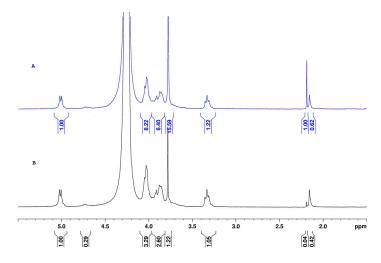
**Figure 6.** As spun fibers from the mixture CS/PEO (80/20) dissolved in acidic  $D_2O$  (**A**); Stabilized and washed chitosan fibers from the mixture CS-102/PEO 80/20 dissolved in acidic  $D_2O$  (**B**).
