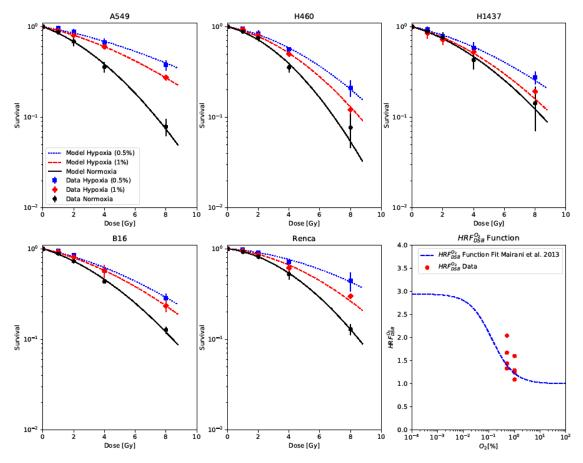
**Figure 1.** Cell survival data of five cell lines irradiated under normoxia (black) and under two hypoxia levels (0.5% and 1% [ $O_2$ ], blue and red) fitted by the model. Lower-right panel: The derived  $HRF_{DSB}^{O_2}$  values compared to a parametrization introduced in [11].
