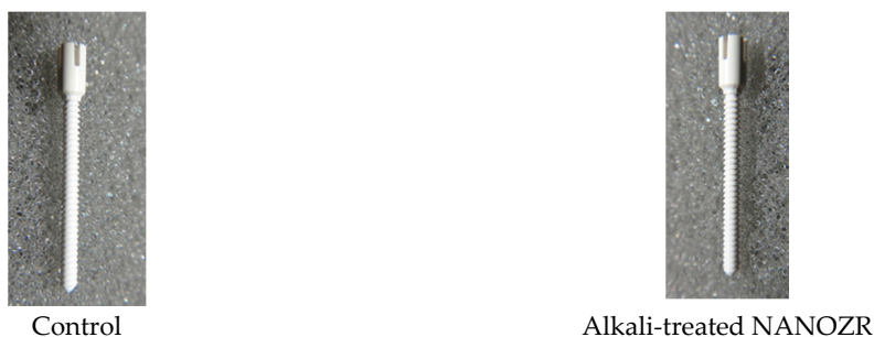
Figure 10. The control and alkali-treated NANOZR implant photographs.
