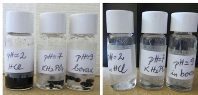
Figure 4. MWNT-DNA-CTAB and PEG-DNA-CTAB gel particles in different pH solution after one week.
