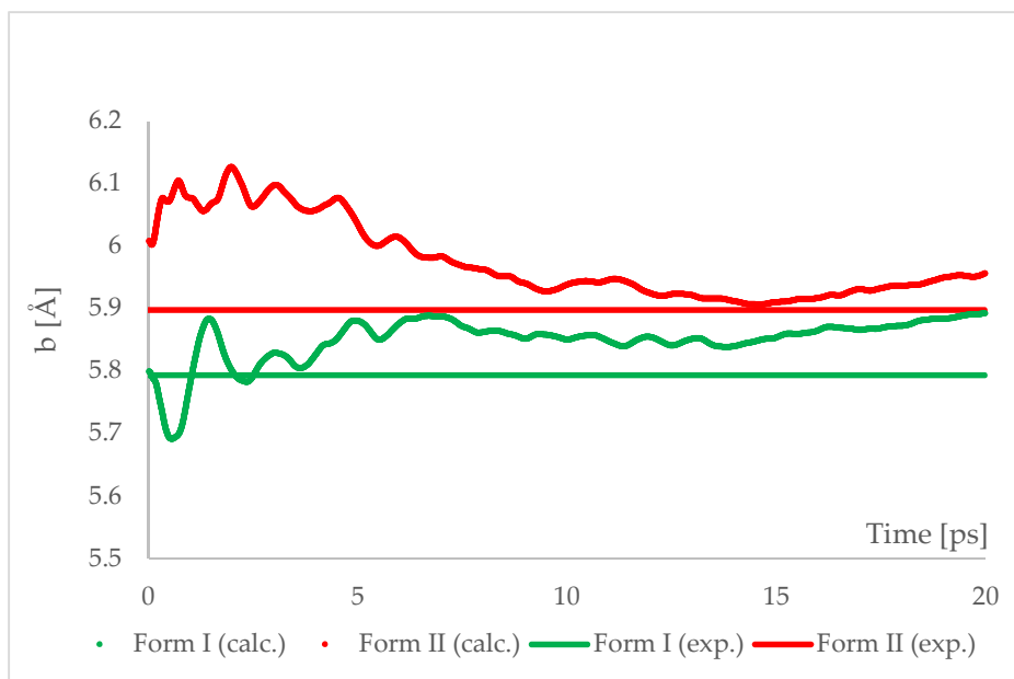
Figure S1. Running average of the unit cell length “b” obtained from aiMD simulation at T=293 K and p=6.2 GPa using PBE TS functional. Horizontal lines represent the experimental values.
