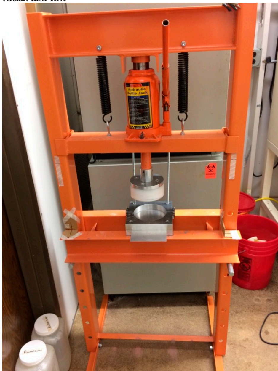
Figure S1: Ceramic disc molding apparatus consisting of a hydraulic press and aluminum disc mold for the formation of ceramic filter discs
