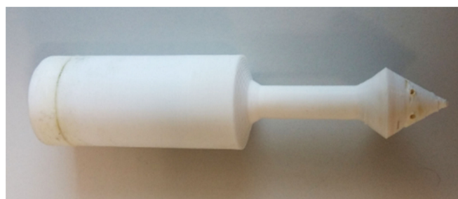
Figure 10. Photo of the PP reactor after the 15th reactor cycle (the reactor was used in 15 successive experiments).
