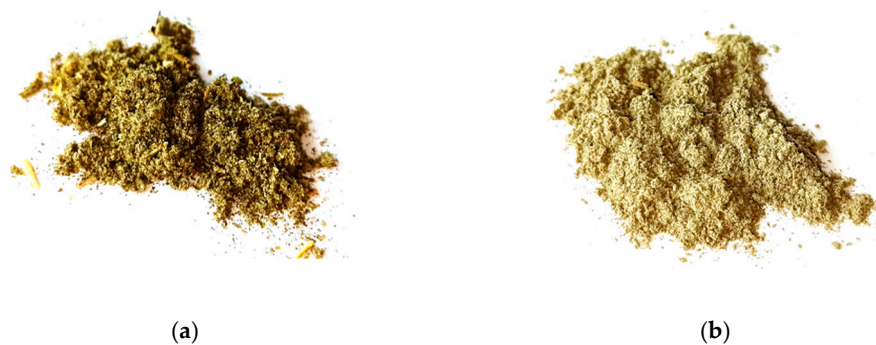
Figure 1. External morphology of (a) unmodified salvia filler (SO filler), and (b) montmorillonite (MMT)-modified SO filler.
