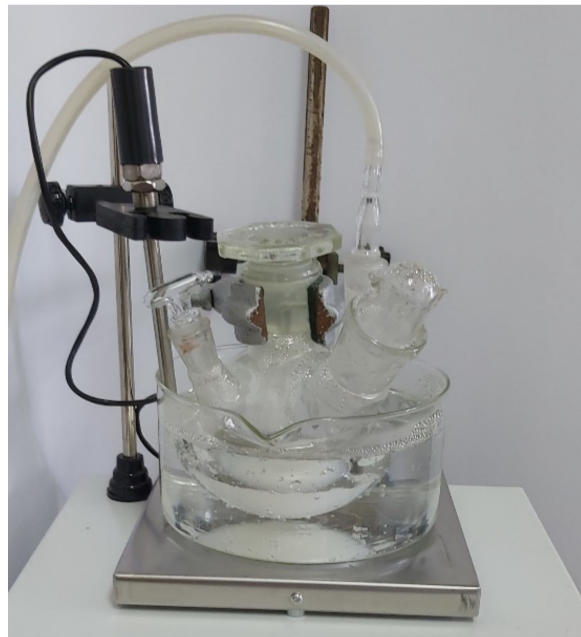
Figure 16. Apparatus for the synthesis of CMS and Ch in the addition of vanillin.
