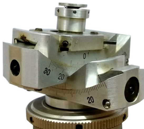
Figure 10. A special goniometer head was designed and manufactured for in situ X-ray studies.
