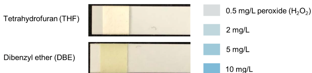
Supplementary Figure S1. The concentration of peroxide in tetrahydrofuran (THF) and dibenzyl ether (DBE). The deeper color means a higher concentration of peroxide.
