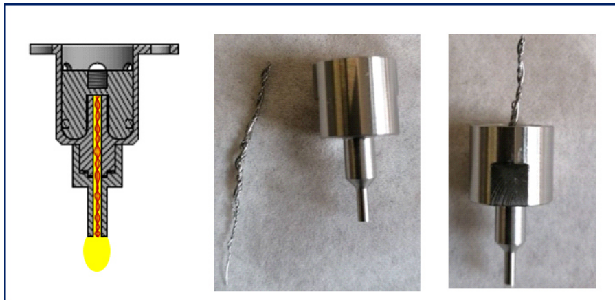
Figure S2: Left: Schematic representation of the twisted wires in the cannula, middle: Photo of the twisted wires and the cannula and right: Photo of the twisted wires inserted into the cannula.
