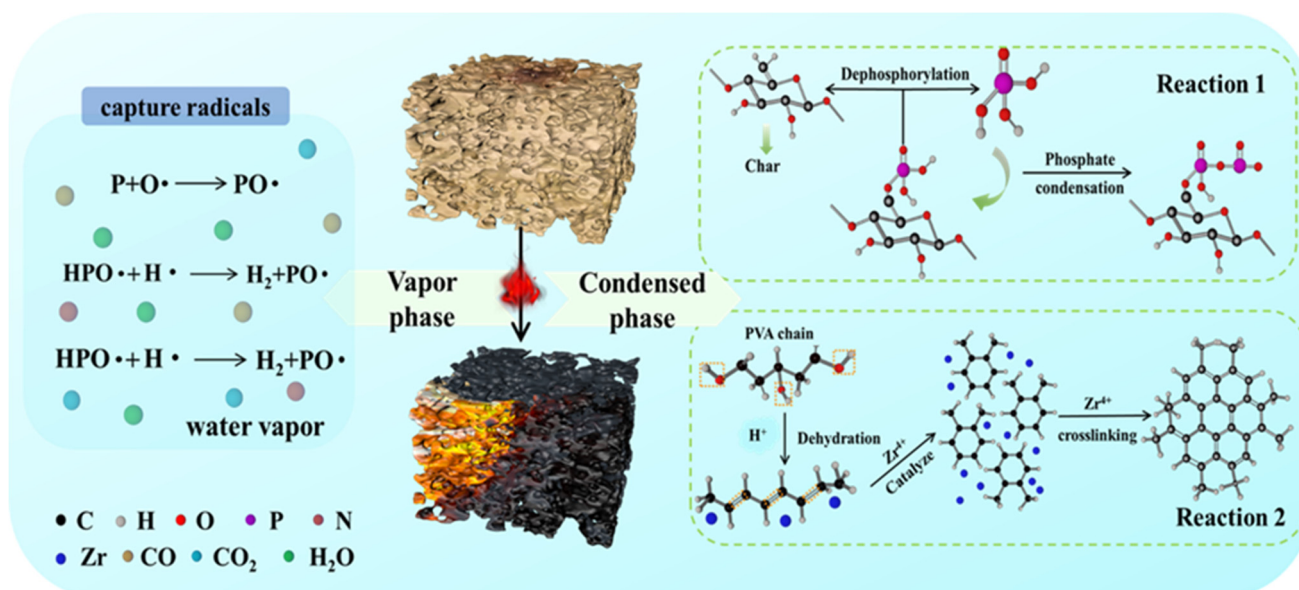
Figure 15. Mechanism of flame-retardancy of PVA/PCF 10 /α-ZrP 10-3 .
