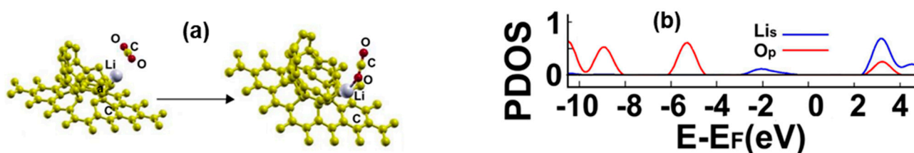
Figure 12. (a) The adsorption of CO_2 on the Li-doped graphene- C_{30} system for the pentagonal base. The initial distance between the carbon atom of the CO_2 molecule and the Li atom was 3.17 Å, and the distance from the graphene layer was 7.12 Å. The molecule was parallel to the graphene layer. The adsorption is without dissociation. (b) The PDOS for the adsorption of CO_2 on the Li-doped graphene- C_{30} system for the pentagonal base.
