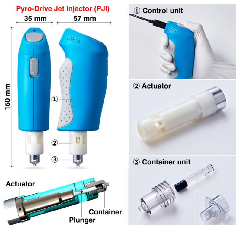
Figure 3. A diagram of the needle-free pyro-drive jet drive injector (PJI), called the Actranza™ lab (Daicel Corporation, Osaka, Japan, https://www.daicel.com/en/business/new-solution/actranza/ , accessed on 1 April 2023). The PJI, which is composed of control unit, actuator, plunger and container, can successfully control two types of gunpowder with different times, weights and burning rates for the adjustment of the sample volume, the penetration depth and wide dispersion of delivery [42].
