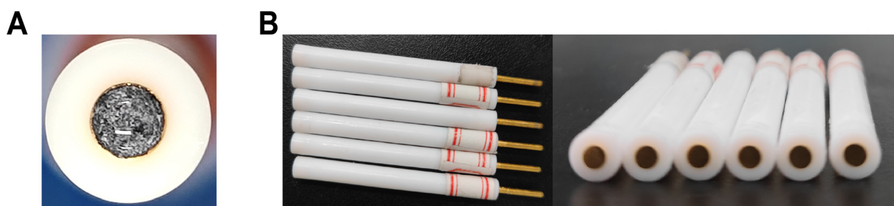
Figure 7. Appearance of E-apt sensor (A). Gold electrodes modified with nanomaterials; (B). The appearance of gold electrodes.
