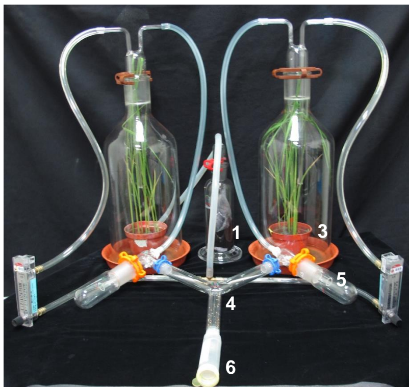
Figure S3. Y-maze olfactometer.
