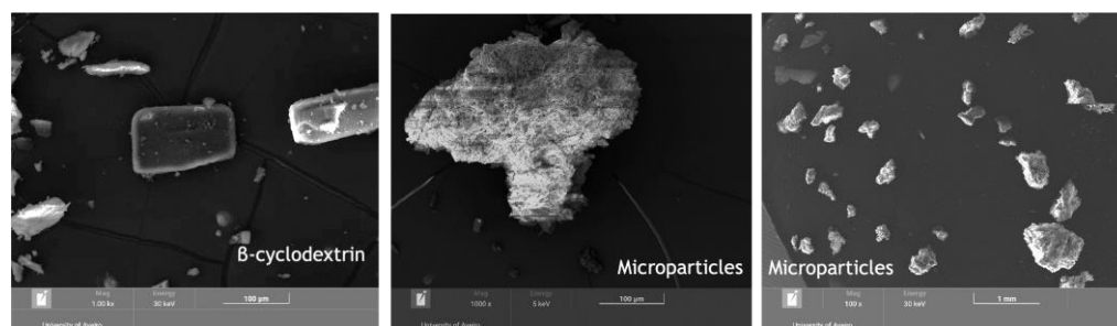
Figure 4. Results of the \beta -CD powder (coating agent) and OP extract microparticles analyzed by scanning electron microscopy (SEM).
