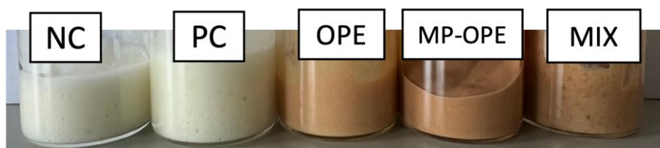
Figure 7. Sunscreen formulations produced for this study. NC—negative control formulation; PC—positive control formulation; OPE—onion peel extract formulation; MP-OPE—microencapsulated onion peel extract formulation; MIX—mixture formulation.
