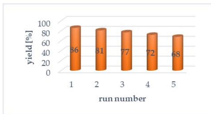
Figure 2. Reuse of the Novozym 435 catalyst.
