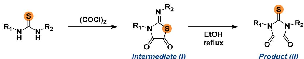
**Scheme 2.** Reaction of disubstituted thiourea and oxalyl chloride.
