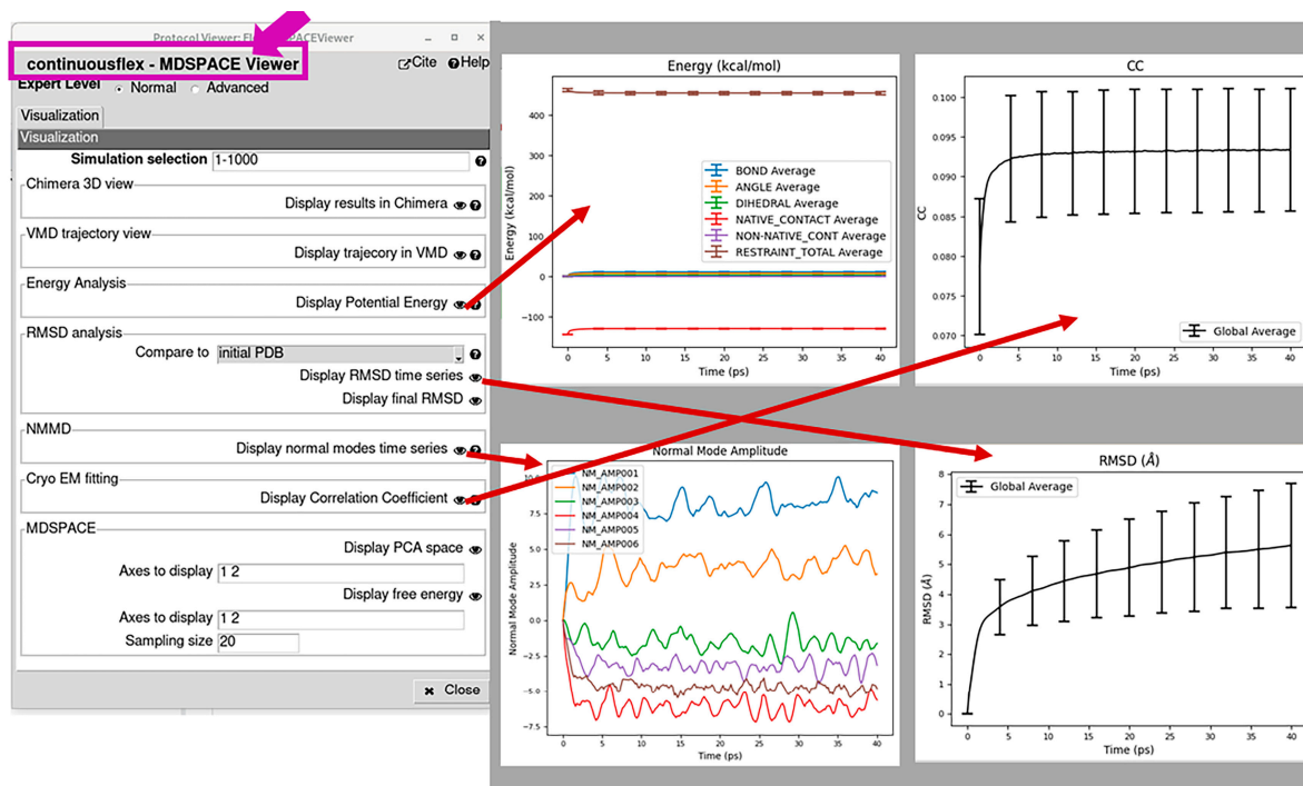
Figure 4. Analysis of the results of data analysis using NMMD simulations (corresponding to the “MDSpace”/“MDTOMO” box in Figure 1B,C). The viewer allows a statistical analysis of the energy, correlation coefficient (CC), normal mode amplitudes, and root mean square deviation (RMSD) trajectories over a selected set of particle images or subtomograms (“Simulation selection”). Also, for one selected particle image or subtomogram, it allows displaying not only these trajectories individually but also the initial and final 3D structures with ChimeraX (“Display results in ChimeraX”) and animating the trajectory of atomic coordinates with VMD (“Display trajectory in VMD”). Note that the results shown in this figure are our arbitrary choice. More precisely, they come from an analysis of 1000 synthetic single particle images using one iteration of MDSpace. Thus, the bars in the CC plot show the standard deviations from the average obtained for 1000 simulations (one simulation per particle image) over the simulation length. In this CC plot, similar standard deviations over the simulation length mean relatively stable simulations. The normal-mode amplitude plot presented here shows the amplitudes of different normal modes during one simulation (for only one particle image, whose index can be specified in the field “Simulation selection”).
