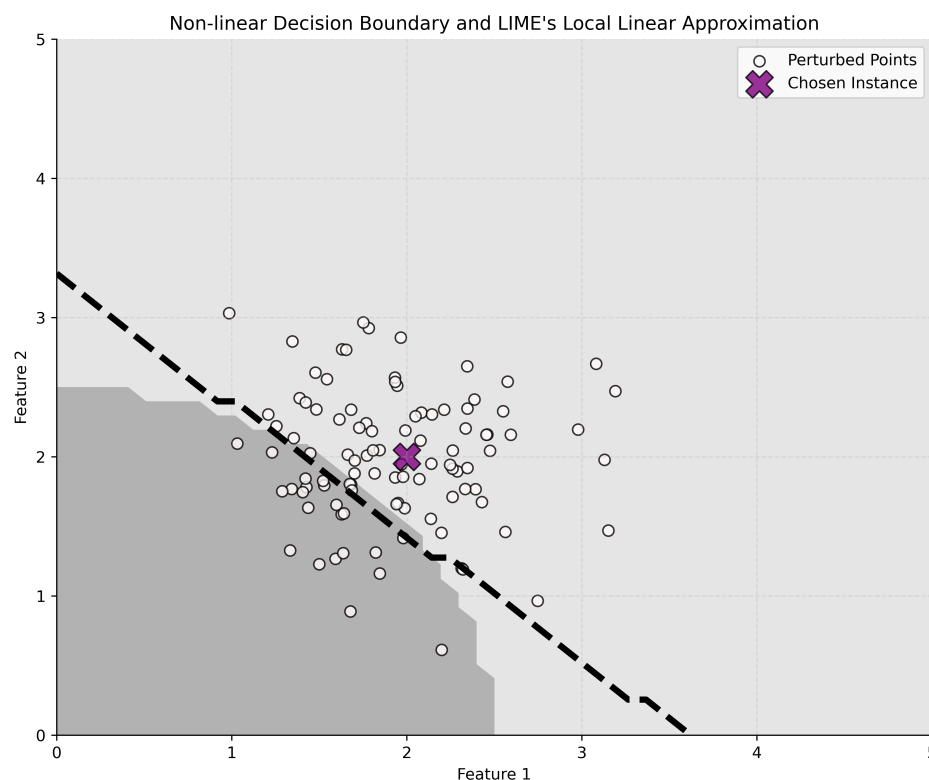
Figure 14. Illustration of how LIME approximates the nonlinear decision boundary of a model (delineated by shades of gray) with a simpler, linear boundary (dashed black line) in the vicinity of a specific data point. The white dots are the perturbed data points sampled around the chosen instance, which is marked in purple.
