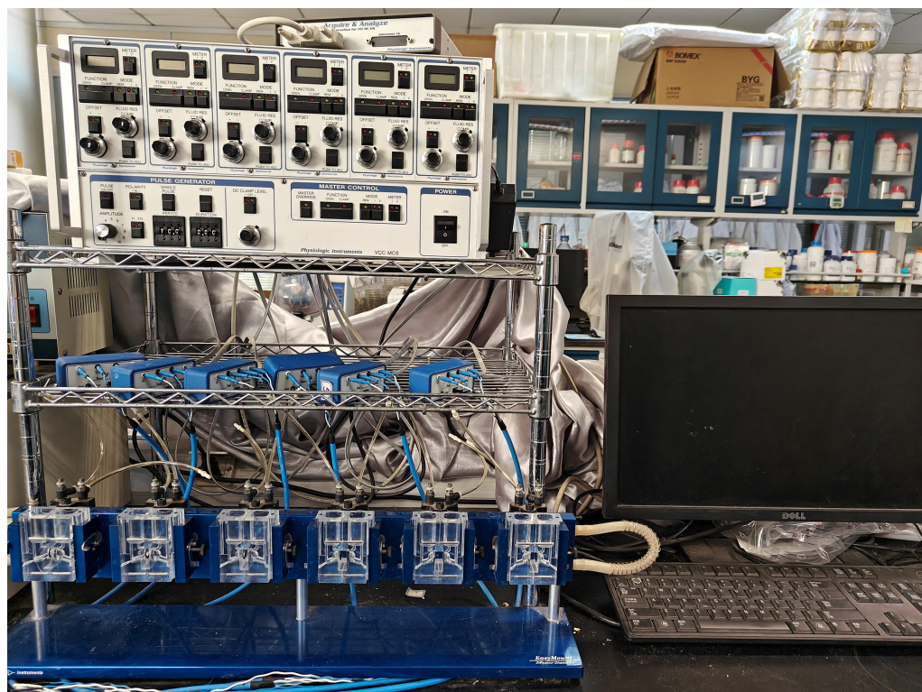
Figure 6. A photo of the Ussing chamber system used in this study.
