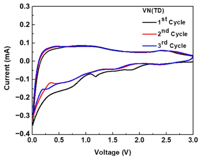
**Figure 9.** Cyclic voltammetry curves of VN (TD)/C composite electrode synthesized by the thermal decomposition of vanadyl phthalocyanine.
