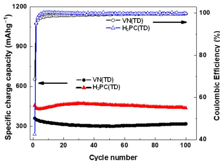
**Figure 10.** Specific discharge/charge capacity vs. cycle number Coulombic efficiency of VN(TD) and H<sub>2</sub>PC(TD) electrodes after 100 cycles at 100 mA g<sup>-1</sup>.
