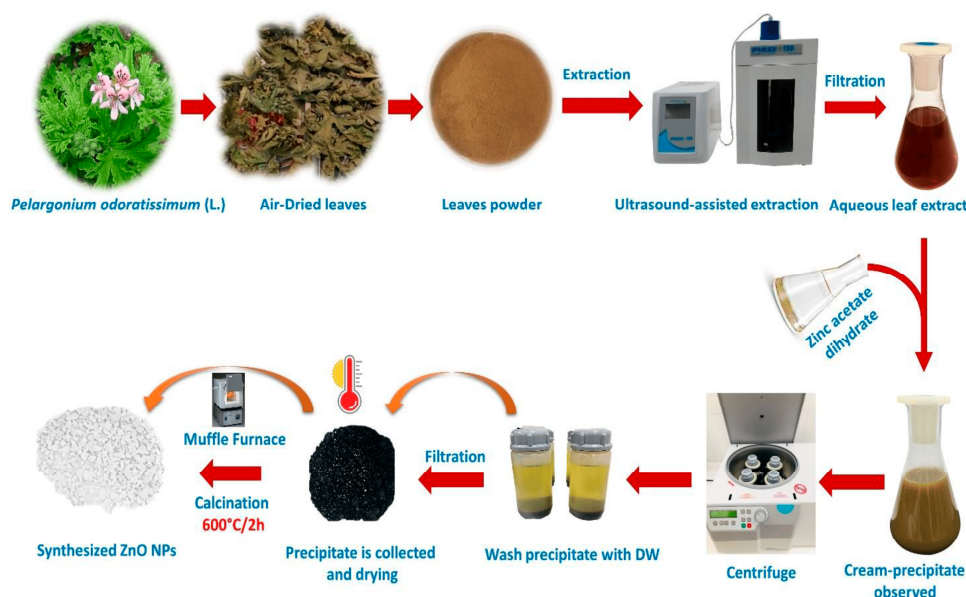
Figure 2. A graphical representation of the green synthesis of ZnO NPs using an aqueous plant extract. Figure reuse from [27].
