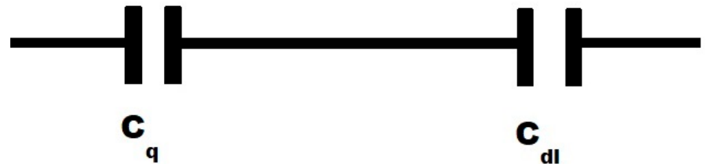
Figure 1. Schematic illustrations of equivalent circuits of C_{int} .
