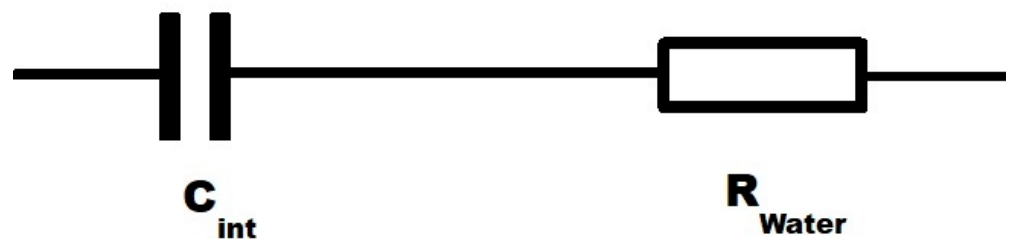
Figure 3. Schematic illustrations of equivalent circuits of C_m .
