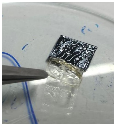
Figure S17. Photograph illustrates the process of the removal of the PPC film from the matrix of PPC /PIL-10 (1/1 wt/wt) on Si wafer.
