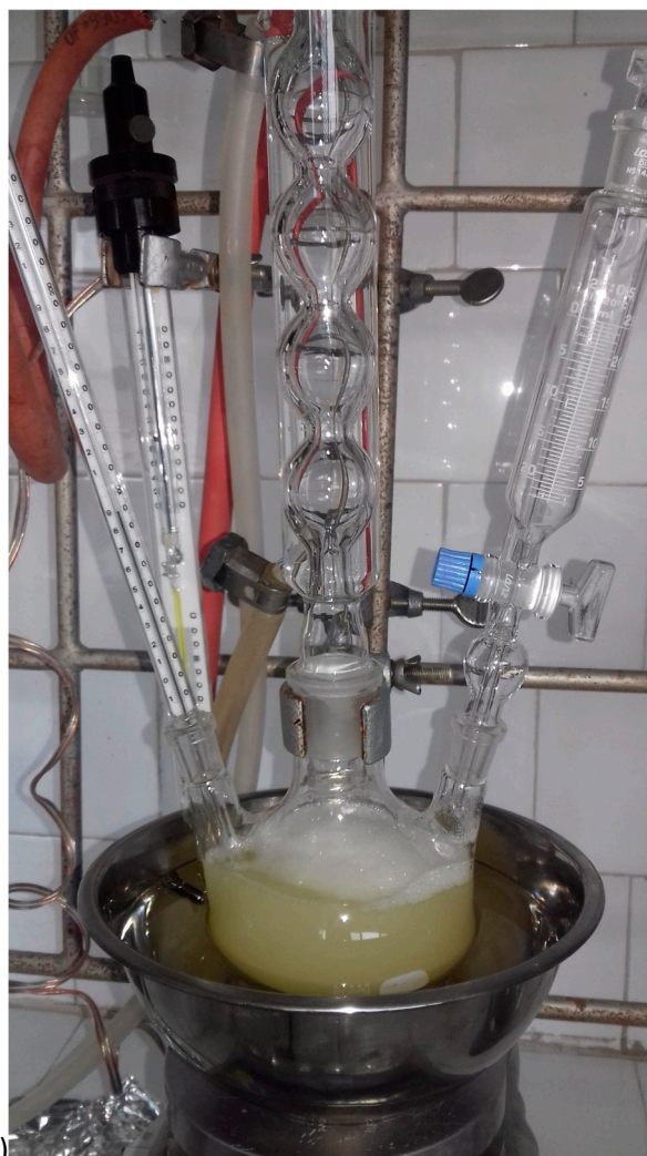
Figure S2. Alkylation installation a) Cooling bath, b) heating bath, photo Iuliana Vasian
