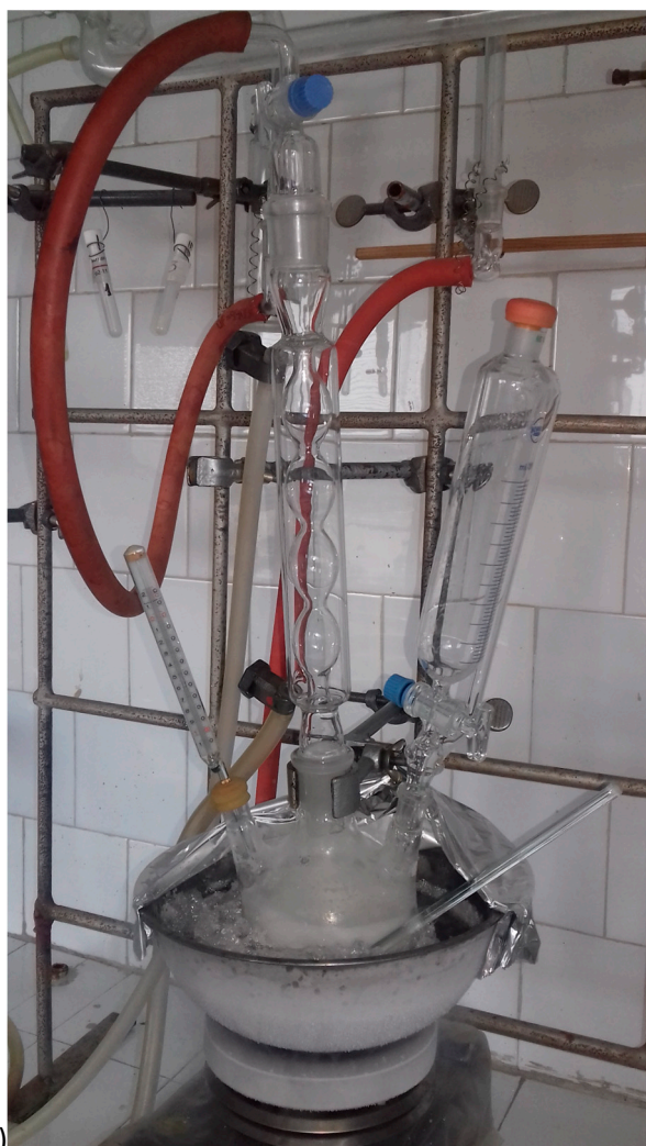
Figure S2. Alkylation installation a) Cooling bath, b) heating bath, photo Iuliana Vasian
