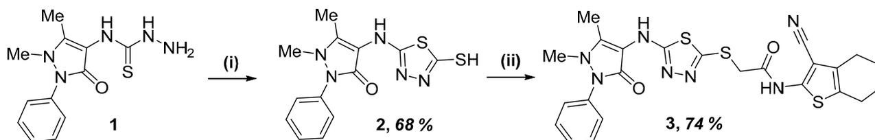
**Scheme 1.** Synthesis of title compound **3**. Reagents and conditions: (i)—**1** (10 mmol),  $K_2CO_3$  anhyd. (5 mmol),  $CS_2$  (10 mmol), ethanol (15 mL), reflux 4 h; (ii)—**2** (10 mmol), KOH (10 mmol), 2-chloro-*N*-(3-cyano-4,5,6,7-tetrahydrobenzothiophen-2-yl)acetamide (11 mmol), KI (traces), ethanol (10 mL), reflux 1.5 h.
