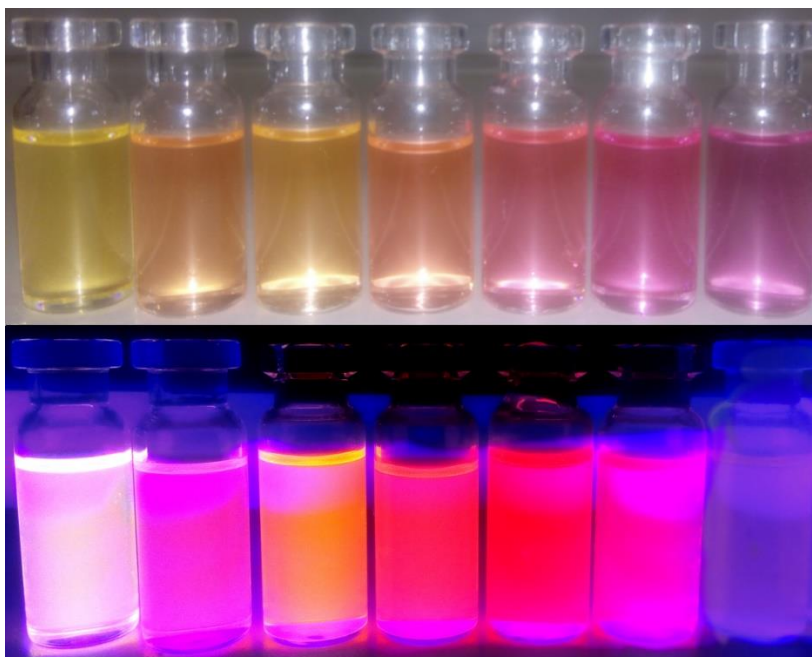
Figure S1. Solutions of synthesized amine 3 in benzene, chloroform, ethyl acetate, acetone, dimethylformamide, dimethyl sulfoxide, and ethanol in visible and UV light (365 nm).
