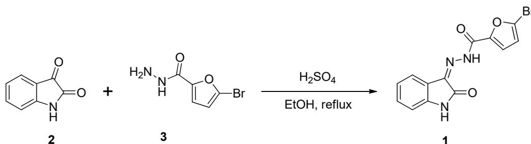
**Scheme 1.** Synthesis of 5-bromo-*N'*-(2-oxoindolin-3-ylidene)furan-2-carbohydrazide (1).
