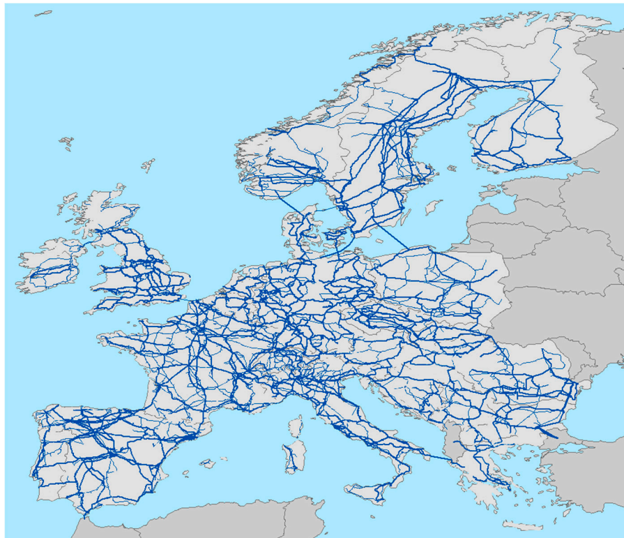
Figure 1. Schematic representation of the transmission line network (220–999 kV) in the European Union. The figure highlights how intensively this area is interconnected through transmission lines.
