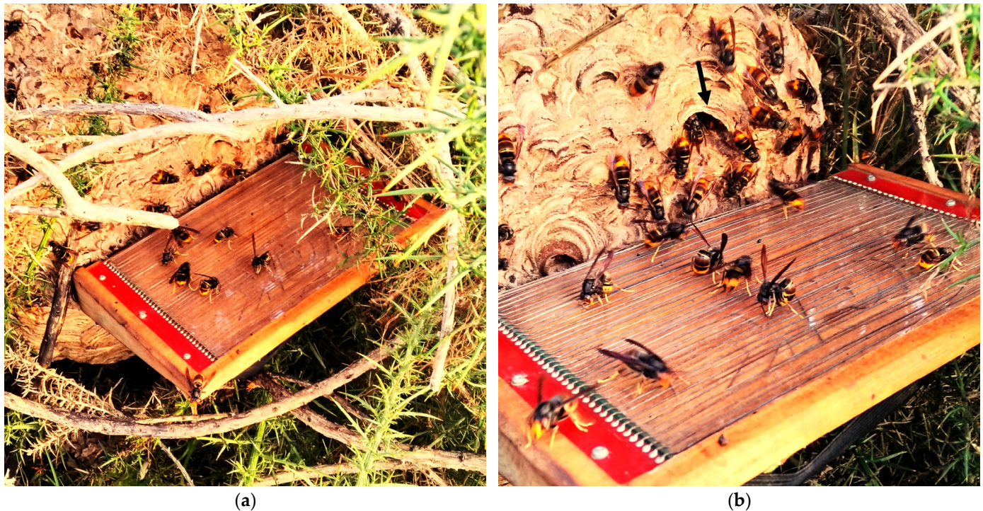
Figure 2. (a) Electro-stimulation device activated and positioned below the lateral entrance of the Vespa velutina nest. This strategic placement facilitates efficient stimulation and venom collection without direct handling, as it interacts with both worker hornets exiting the nest and those returning from foraging. (b) Close-up view highlighting the lateral entrance of the nest, indicated by a black arrow, through which hornets actively engage with the electro-stimulation setup.
