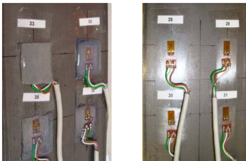
Figure 1. This figure shows instrumented strain gauges on both sides of Specimen 3.
