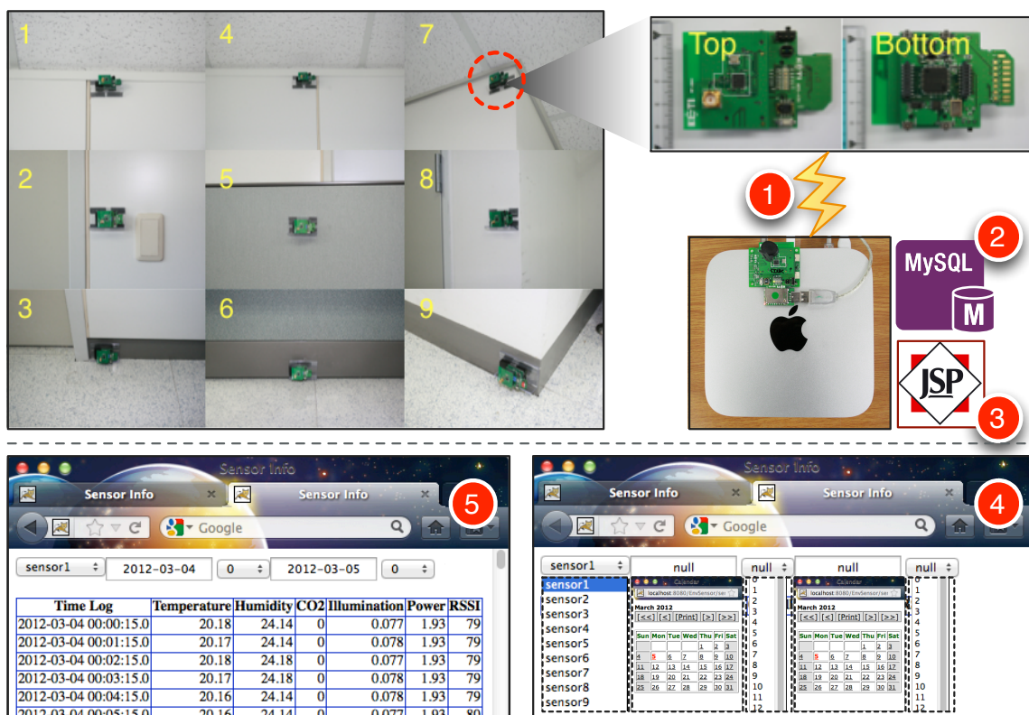
Figure 2. Our experimental setup of nine wireless sensor nodes mounted on our laboratory’s wall. (1) A wireless sensor node transmits captured data to the sink node connected to the Mac mini; (2) a Java-based logging program puts the received data into the MySQL database table; (3,4) a JSP-based Web page provides a user interface for selecting the sensor, the day, the time duration of interest; (5) it retrieves and shows the saved data as a table or graph.
