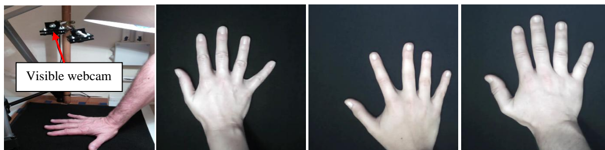
Figure 3. Hand dorsum infrared acquisition system (figure on the left) and examples of acquired IR hand images from different users (three figures on the right).
