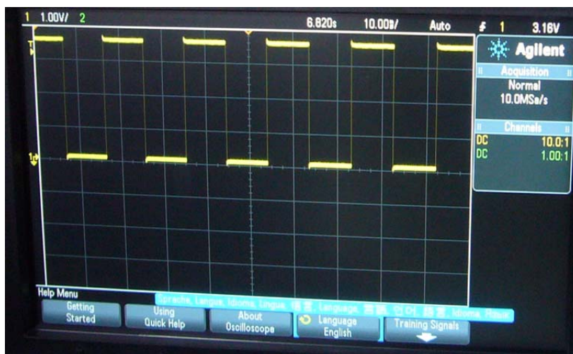
Figure 11. Digital output of the Hall sensor displayed on an Agilent 3032A oscilloscope.
