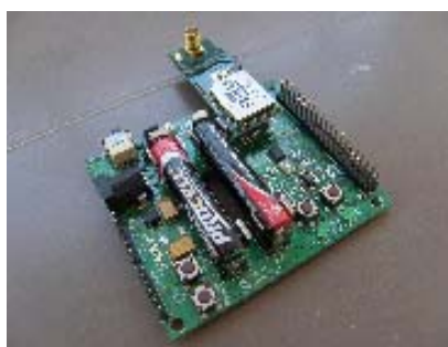
Figure 20. Zigbee sensor board.
