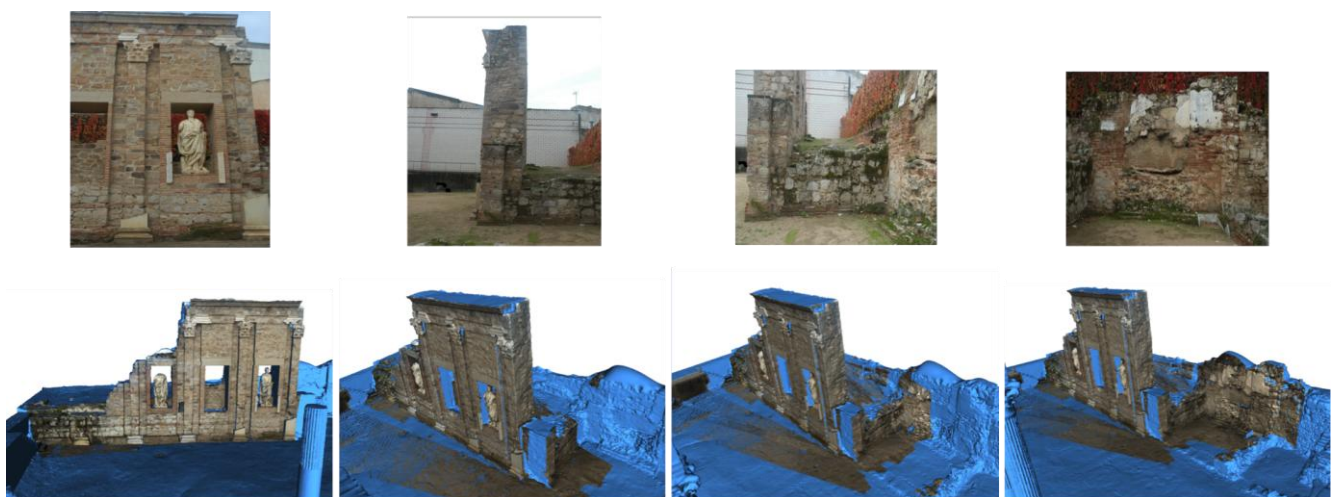
Figure 17. External images taken under appropriate environmental conditions ( top ); Evolution of the coloured model as the colour information is added ( bottom ).
