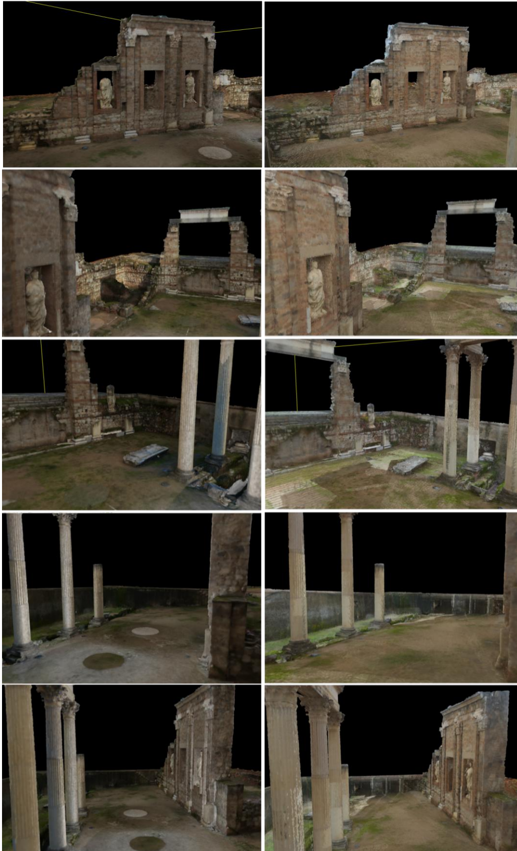
Figure 18. Pictures of a previous coloured model generated from the images provided for the scanner on-board camera ( left ) in comparison with pictures of the photorealistic model created from the geometrical model and a set of external images taken without any restrictions ( right ).
