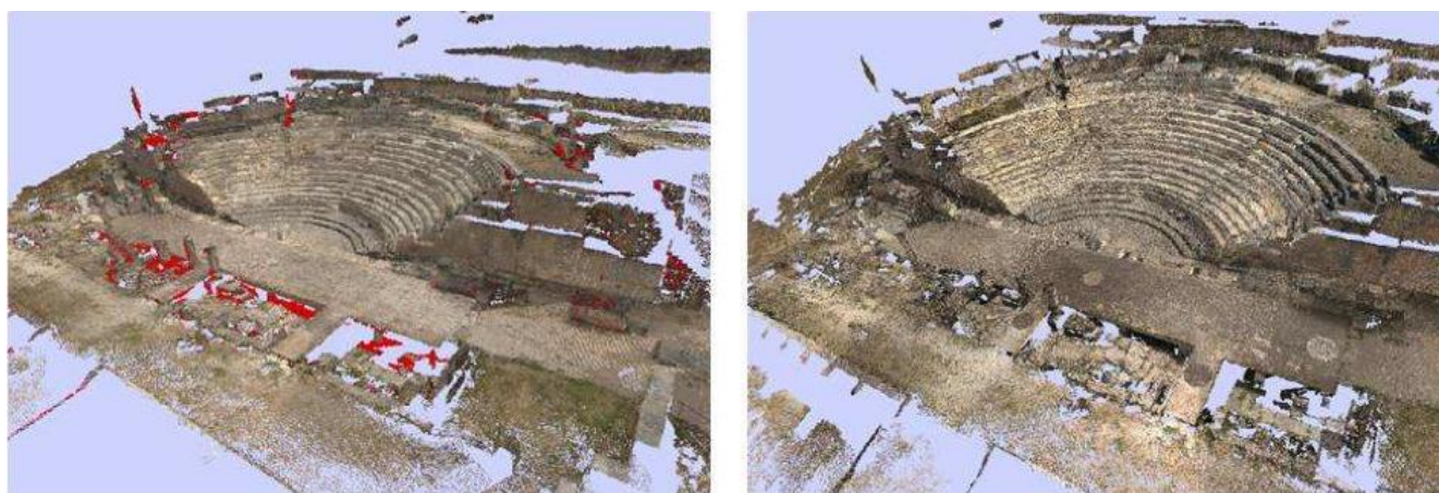
Figure 14. Two views of the final geometrical model for the Fori Porticus of Emerita Augusta.
