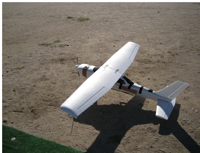
Figure 1. Mentor Multiplex aircraft modified by the authors to be a UAV.
