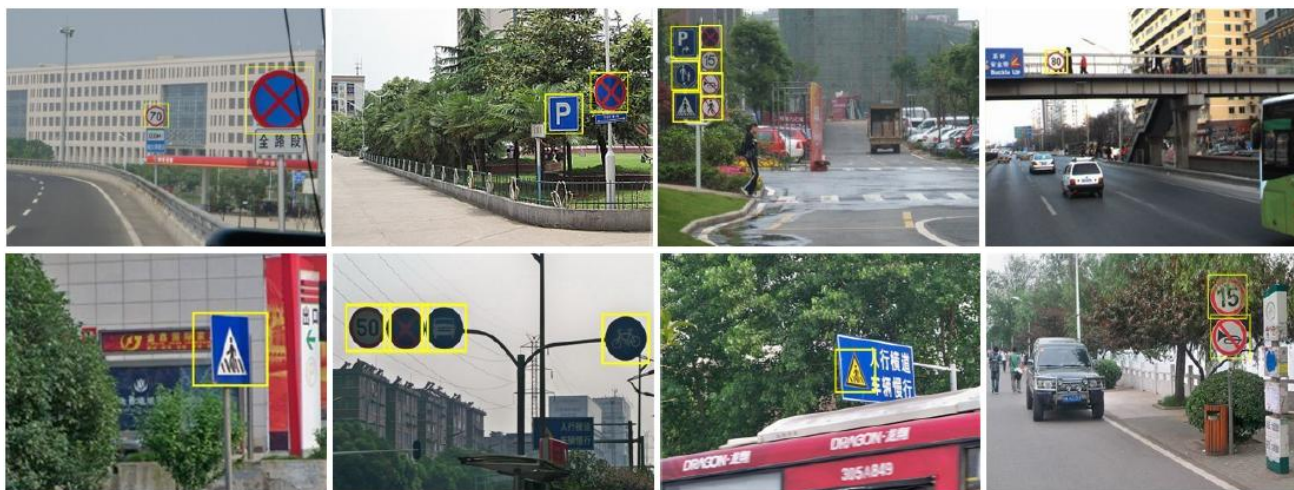
Figure 13. Detection of traffic signs under various conditions.
