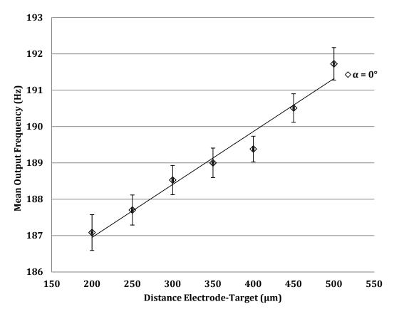
Measurement errors equal  $\pm 1\%$ , which is the same order of magnitude as the previously seen optical method. The response time is however longer due to oscillator ( $\pm 40~\mu s$ ) and filter/buffer processing. Due to the electronics involved, this method is more complicated to implement than the optical
