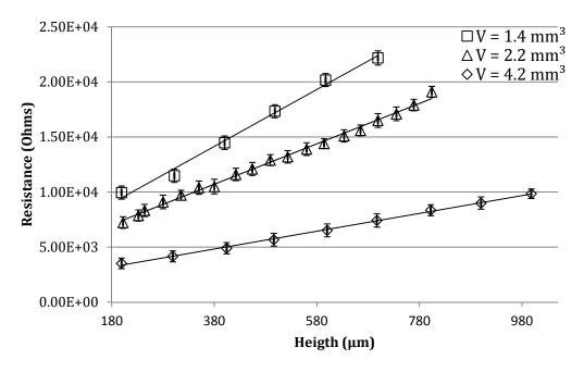
The electrical resistance of droplets is measured for the different volumes of water and for different values of the separation distance between the needle from which the bubble emerges and the top electrode. In the first step, the electrode is placed far from the contact position and the droplet is
