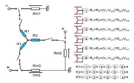
If speed frequency from one circuit to the other is fast enough, the sampled resistances will lead to the platform position because there is a link between the resistance and the geometry. Thus, Figure 3 illustrates the equivalent electrical circuit for the bubbles and the table. If the switching frequency is high enough, the resistance of each bubble and droplet can be determined using the following equation:
