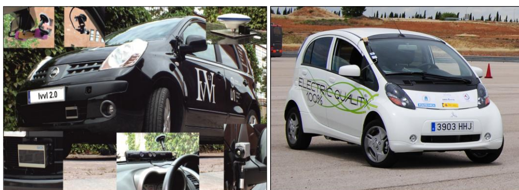
Figure 1. Left platform IVVI 2.0 with all the sensing devices available. Right vehicle with the communication receiver.
