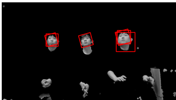
Figure 10. Results from face detection based on Figure 9 and the use of eye detection.
