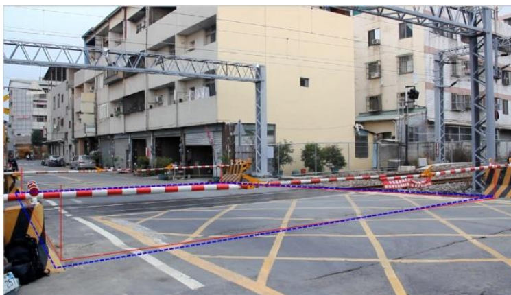
Figure 10. The detection result of the risk area, where the blue-line area is the detection result and the red-line area is the real measured result.
