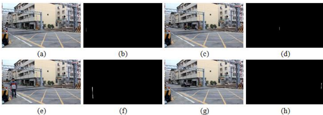
Figure 9. The test object with length 100 cm for the terrain drop compensation: (a) the test rod on rear-left; (b) the extracted test rod image of (a); (c) the test rod on rear-right; (d) the extracted test rod image of (c); (e) the test rod on front-left; (f) the extracted test rod image corresponding to (e); (g) the test rod on front-right; (h) the extracted test rod image corresponding to (g).
