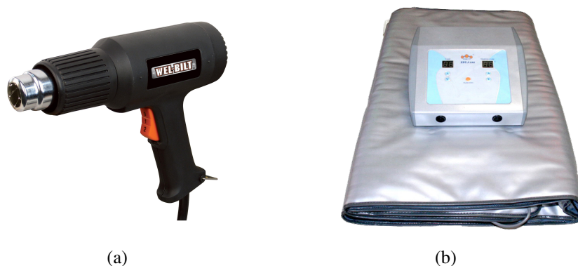
Figure 9. First stimulation tools used in non-destructive testing (NDT) with infrared thermography (IRT). (a) Heat gun. (b) Thermal blanket.
