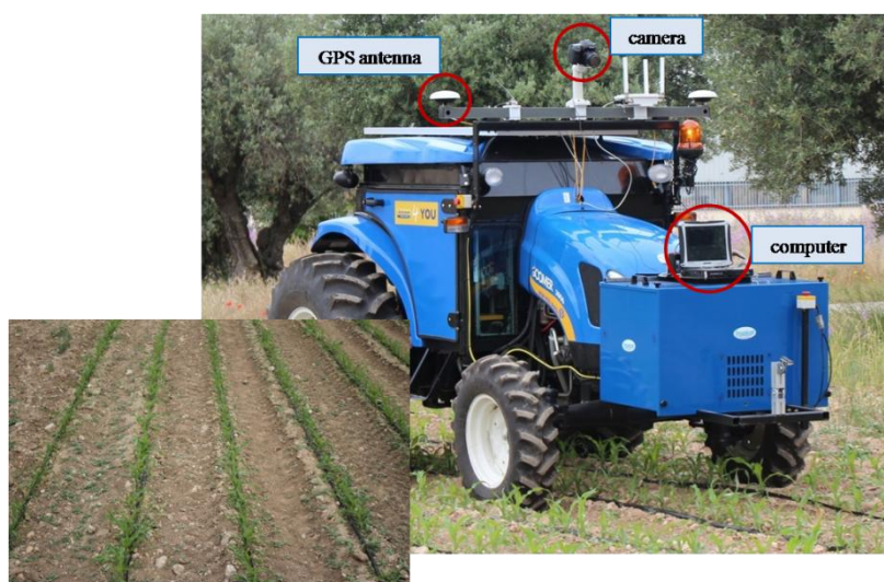
Figure 1. A RGB camera on board an autonomous tractor acquiring geo-referenced images in real conditions (lighting and tractor speed) in a maize crop.
