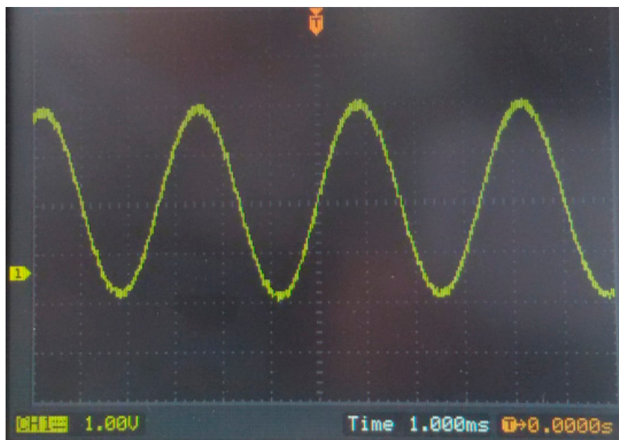
Figure 14. Transient output waveform of the integrated Hall sensor for a 1 kHz 170 mT sinusoidal magnetic flux density.
