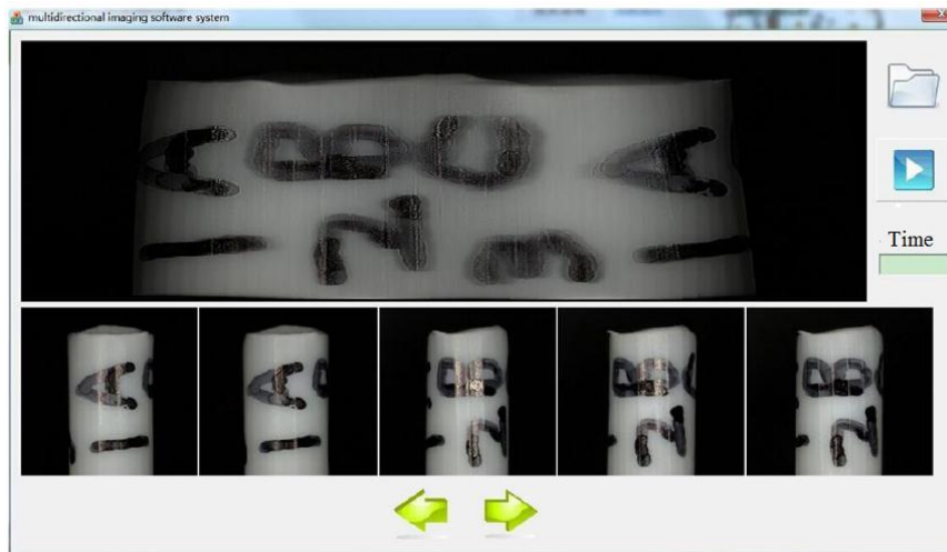
Figure 4. Developed software system to create panoramic image from a series of images taken from different rotation angles.
